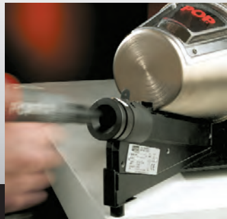
Rivet Presenter speeds up assembly process and improves productivity
